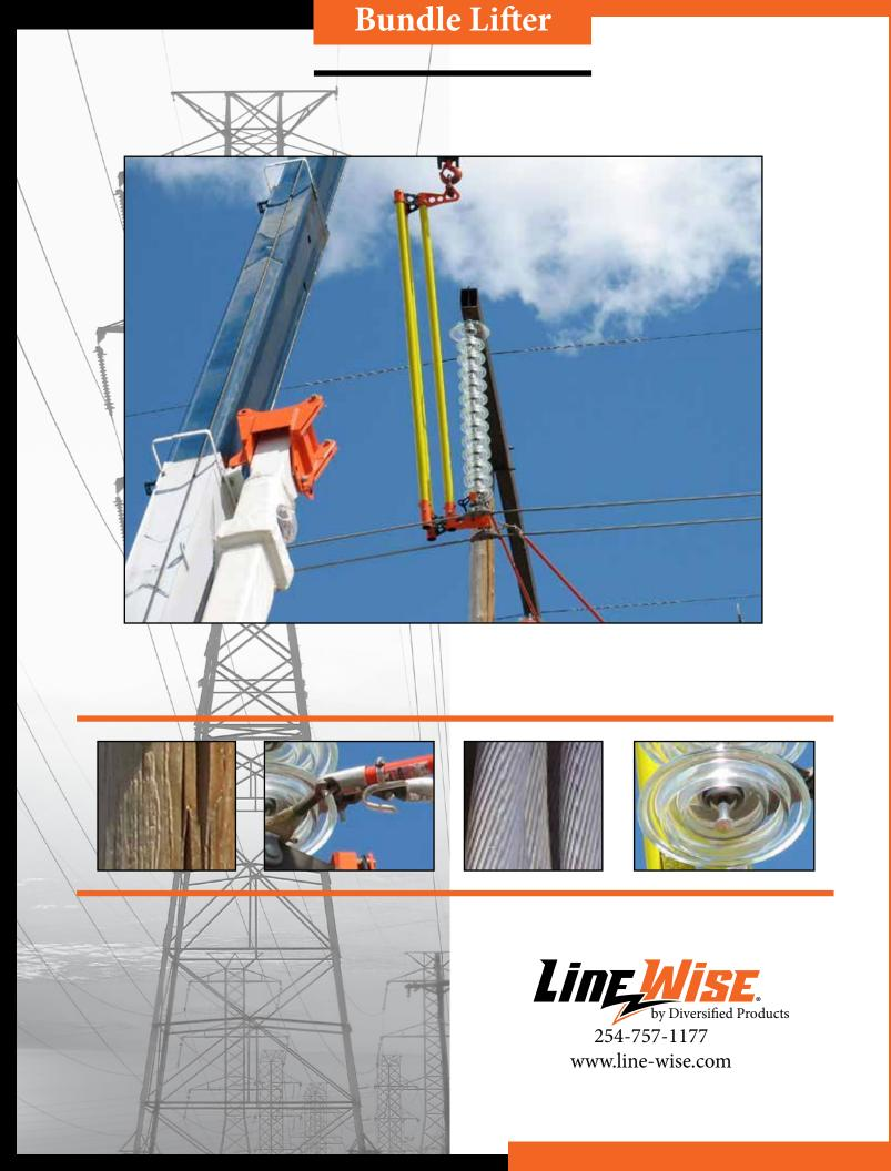
The bundle lifter keeps the yoke plate in a vertical position so the insulator string can be connected easily.
